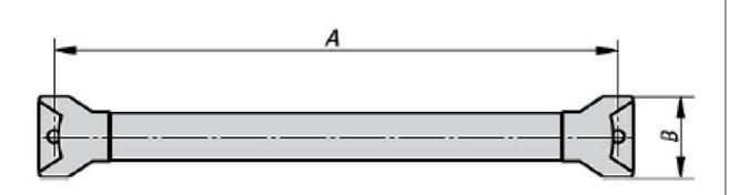
D= 25mm / 0.98 inch T= 3,5mm / 0.13 inch A= 250mm / 9.84 inch B= 43mm / 1.69 inch L= 266mm / 10.47 inch B1= 14,5mm / 0.57 inch L1= 190mm / 7.48 inch H= 65,5mm / 2.57 inch
